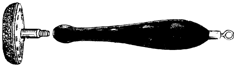
Fig. 1. Sponge-covered metal electrode (attached to the positive pole).
